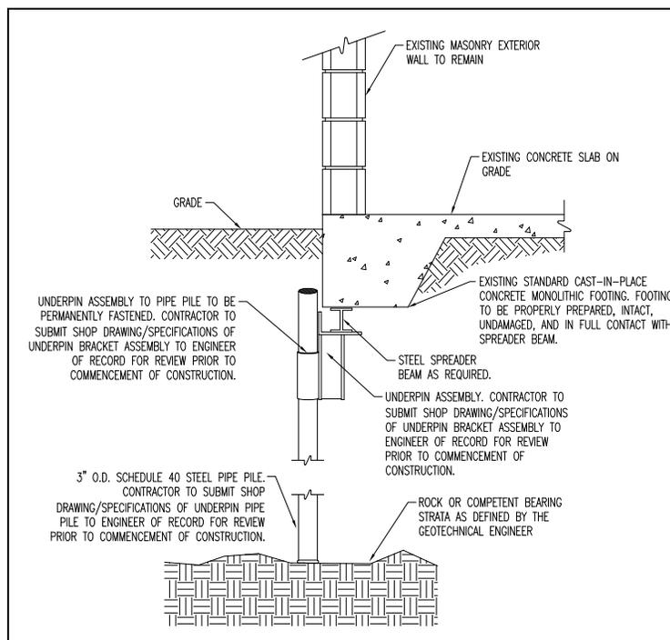
**Figure 2:** Detailed drawing of a typical underpin on a monolithic thickened edge foundation system
