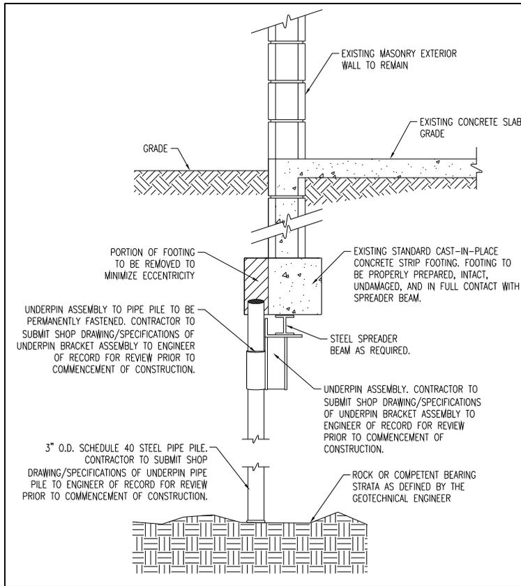
**Figure 1:** Detailed drawing of a typical underpin on an exterior strip footing wall system
