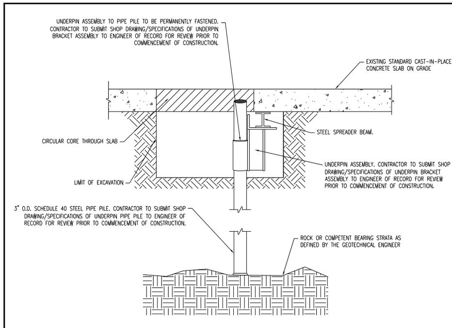
**Figure 3:** Detailed drawing of a typical underpin on an interior concrete slab on grade.
