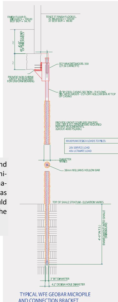
TYPICAL WFE GEobar MICROPILE AND CONNECTION BRACKET
