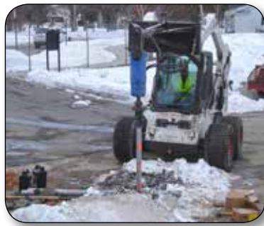
Advancing helical test probe; torque recorded at one-foot intervals
