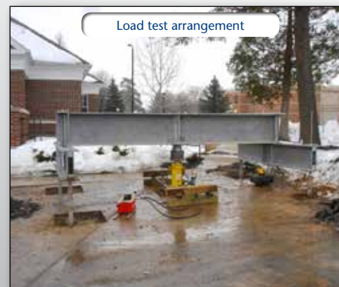
Helical piles advanced; congested working space
