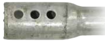
Photo 3: Upset Coupler With Over-Sized, Closely-Spaced Bolt Holes
