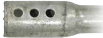
Photo 3: Upset Coupler With Over-Sized, Closely-Spaced Bolt Holes
