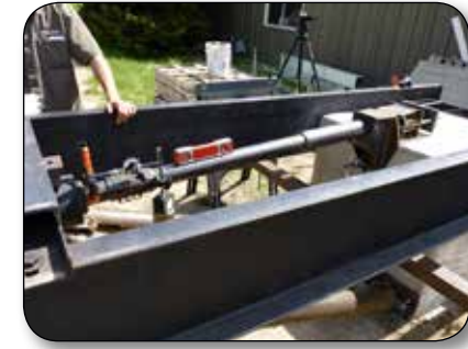
Figure 4: Side-load retrofit system against block of concrete
