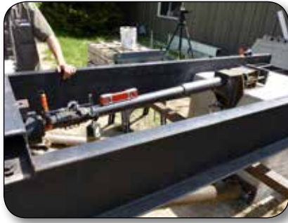
Figure 4: Side-load retrofit system against block of concrete
