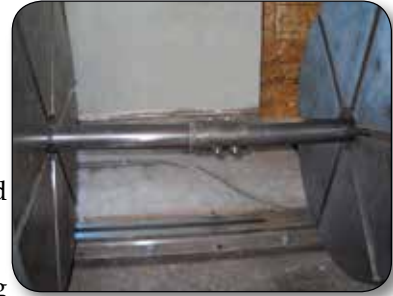
Figure 2: Torsion testing of shaft and coupling
