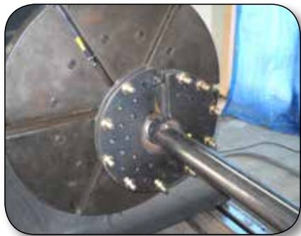
Figure 3: Torsion testing of shaft and helix plate
