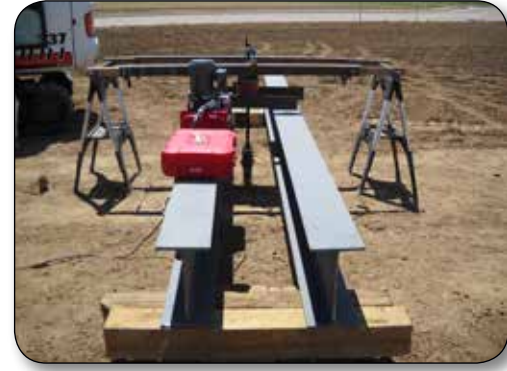
Figure 5: Full-scale field tension test
