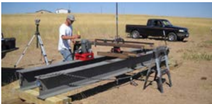
Tension load test
