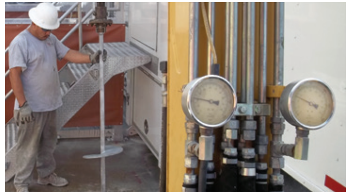
Figure 1: Dual pressure gauges mounted to arm of excavator
