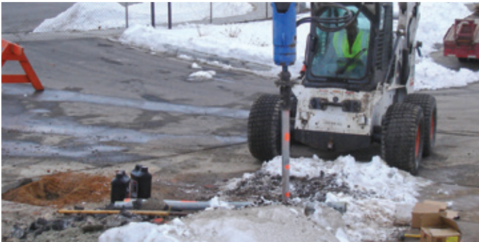
Advancing helical test probe; torque recorded at one-foot intervals
