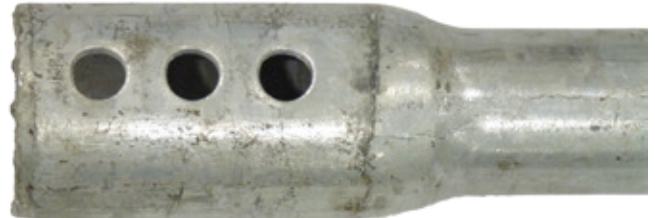
Figure 3: Upset Coupler With Over-Sized, Closely-Spaced Bolt Holes
