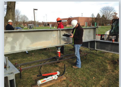
Compression load test
